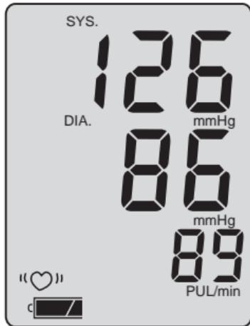
The measurement is stored automatically. If the memory store is full (90 measurements), the oldest measurement is deleted and the current one stored.
