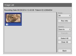
To switch between video and still image thumbnail display, use the ♠, ♣, ♠, and ▶ buttons to select the [Display] box, and press the ENTER button.
