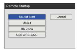
When [USB 4] or [RS-232C] is selected, the remote system's on/off operation will be linked to that of the unit via the selected connector.
