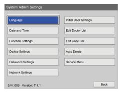
The setting screen for the selected item appears. The serial number of the unit and the current software version appear at the bottom left.
