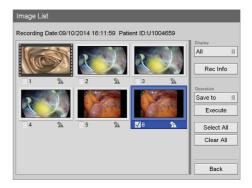
5 Use the ♠, ♣, ♠, and ▶ buttons to select the [Operation] box, and press the ENTER button.
