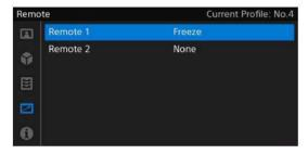
3 Select the functions to use with the foot switch, and then press the SET button.
