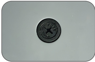
The fuse is located on the bottom of the device
