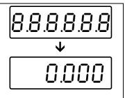
Should the balance not display exactly zero despite empty weighing pan, press the
