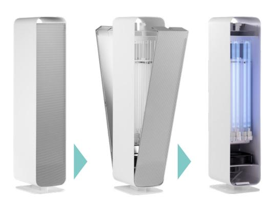
UV-C STERILON FLOW 72 W and UV-C STERILON FLOW 144 W luminaires are equipped with removable covers for fluorescent lamps. Thanks to this, after their removal, the luminaire can be used for direct disinfection (one- or two-way). All safety rules regarding the use of direct floodlights emitting ultraviolet light should be observed, and in particular no one should be in the disinfected room.
