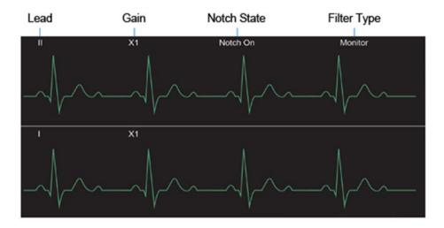
Figure 7-3: ECG wave in normal display format
