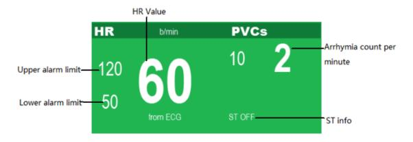
Figure 7-4: ECG parameter in standard display format
